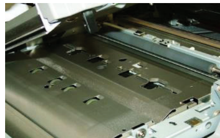
A Registration Gate de-skews the paper and then drops as the sheet advances to the Contact Image Sensor for additional adjustment.
