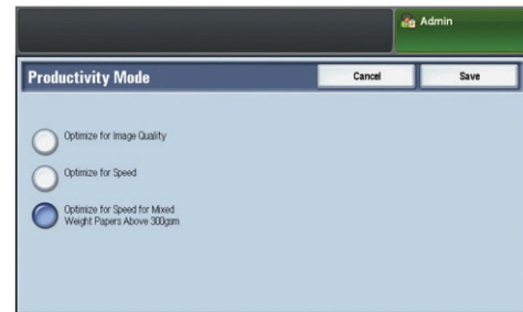
The Versant® 3100 has a third setting: Optimize for Speed for Mixed Weight Papers Above 300 gsm.
