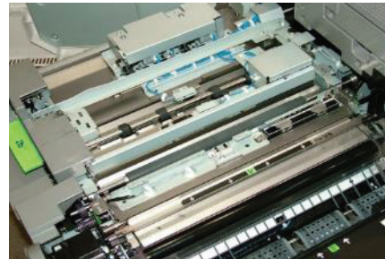
The Aligner Transport helps register the paper to +/- 0.5 mm.
